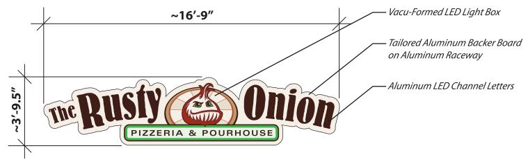
Front-Lit, Plex-Face Channel Letters w/ Backplate & LED, Raceway Mounted
